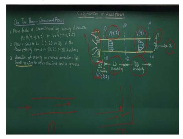
When you talk about any flow systems that flow is having a three dimensions okay. Like as you know it the any velocity, it will have the three components what will come it the  $V_x$ ,  $V_y$ , and the  $V_z$ . It will have the time components in a Cartesian coordinate system. In case of cylindrical coordinate systems, you will have a velocity will vary in a with respect to radius,  $\theta$ , and the z.
