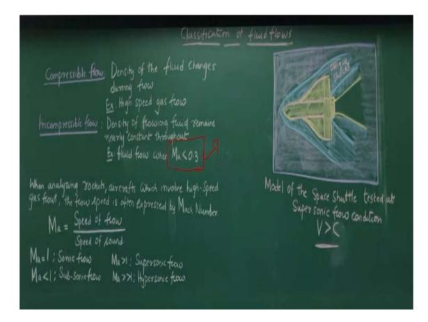
The next concept is that when you talk about a fluid flow systems and as I talk about that density is a mass of the fluid per unit volume. And as you go for a very high pressure zones, high velocity zones okay, there could be a change of the density, either the mass or either the volume will change it so that the density will change it. If it is the density changes, we call the compressible flow.
