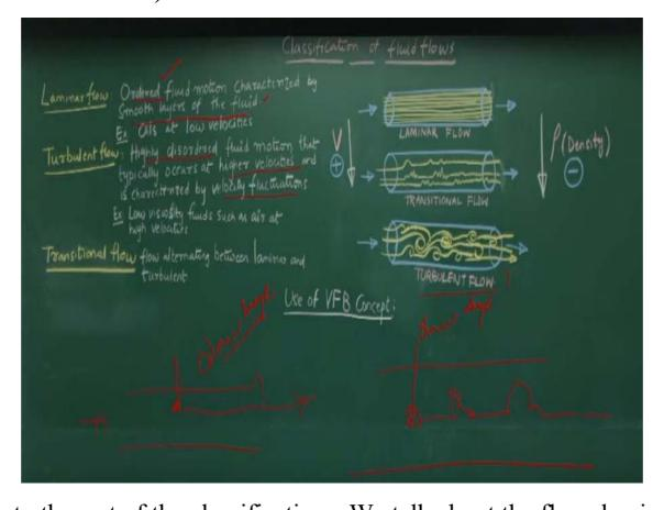
So let come to the rest of the classifications. We talk about the flow, laminar flow, the turbulent flow, and transitional flow. In this case, we consider whenever flow is laminar that means the flow is moving in a smooth layers and they follow very orderly fluid
